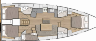
OCEANIS 46.1 - layout 4 CABINS & 2 HEADS
